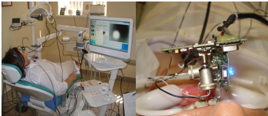
Figure 3. Installation recording the skull bones mobility: A. A general view, B. A close-up view.
